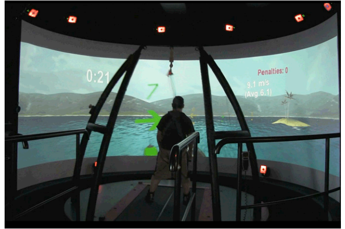
FIGURE 2. Photo of a vestibular subject steering a boat through a slalom course on the CAREN. Wave height, platform movement, and maximum boat speed can be set by the CAREN operator. In this application, the subject must maneuver through the course as fast and with as few errors (e.g., hitting buoys) as possible. © Naval Health Research Center. Reprinted by permission.
