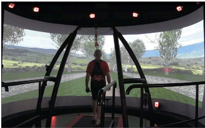
FIGURE 1. Photo of a vestibular subject walking on the CAREN on an endless pastoral path. In this application, the subject sets his own walking speed by pressing up and down buttons on a wireless hand controller. © Naval Health Research Center. Reprinted by permission.
